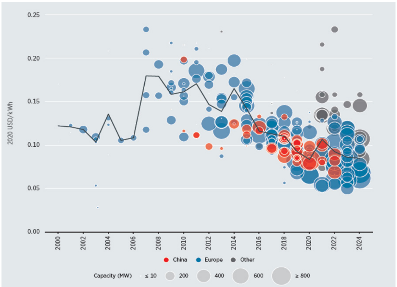
Figure 2 - Levelised cost of energy (LCOE) and auction/power purchase agreement (PPA) prices of offshore wind projects (with global weighted average (black line), 2000-2025 (Source: IRENA, 2021a)
